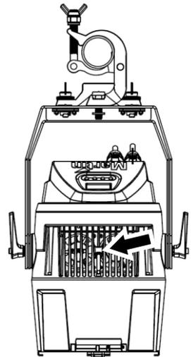
Do not simply loop the safety cable around the legs of the mounting bracket, as this will leave the fixture unsecured if the fixture separates from the mounting bracket.
