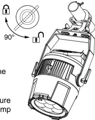
4. Working from a stable platform, hang the fixture with its clamp on the truss and fasten the clamp securely.
