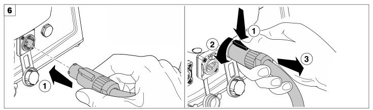
Connecting and disconnecting power cable - Fig. 6
