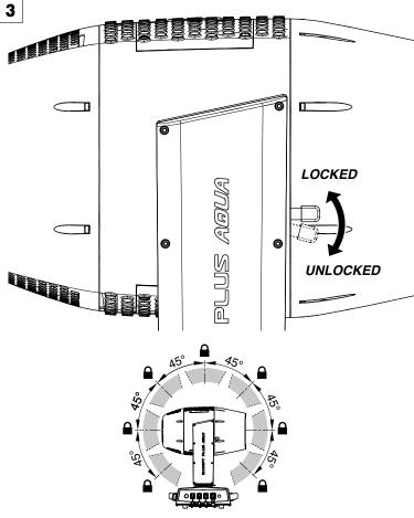
PAN Mechanism Lock and Release (every 90°) - Fig. 2
