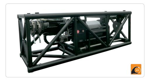
Movecat VMW-S 125-3-30 high-speed winch for universal use in entertainment, tour and events applications. The VMW-S 125-3-30 is tested in accordance with BGV C1 / DGU V 17. DIN 56950-1 and DGUV Principle 315-390 and approved for use above people and in manned airframes as well as conforming to EN 61508 SIL 3. It is capable
