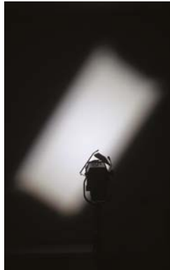
PROPER LIGHT BEAM SHAPING WITH BARNDOOR
